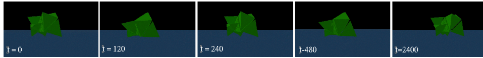
Figure 15: Frames from a video of the evolved locomotion. Cyclic changes in stiffness affect the “leg” on the left, and ratchets the rest of the body to the right.
