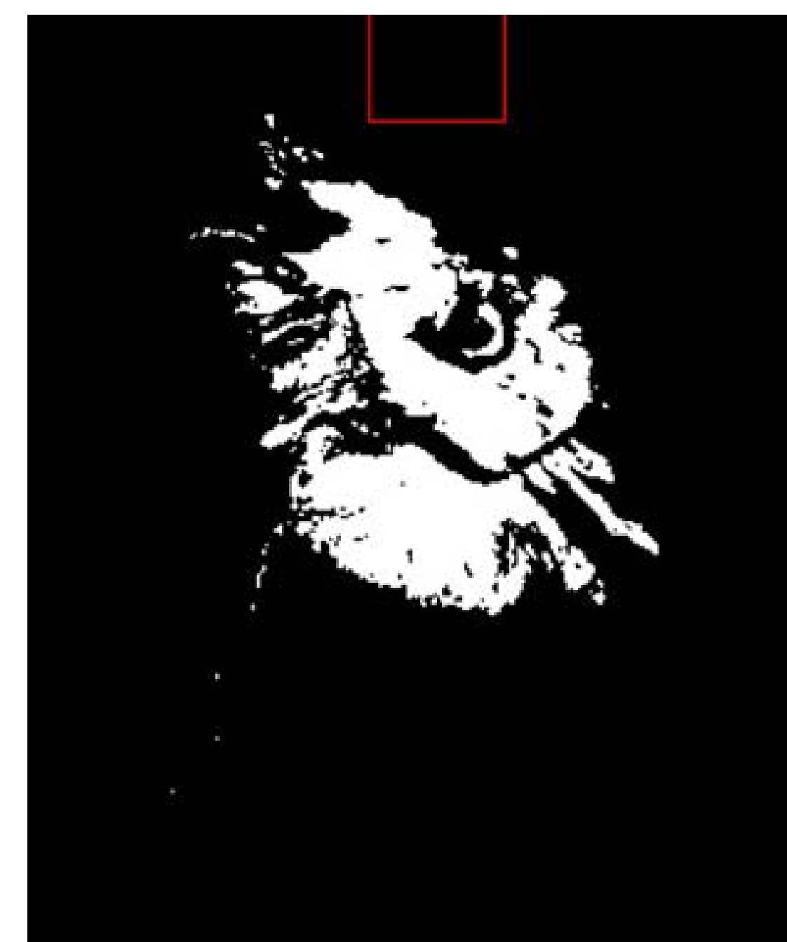
Post classification combination from 12 classes to two classes on snow and rock
