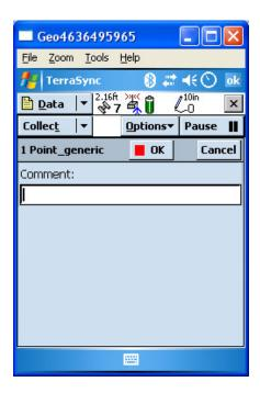
Aim the laser at the feature you wish to offset. Press and hold the Fire Button. When you see a value for distance in the display let go of the Fire button. If your offset values look correct tap on OK. If they do not look correct aim at the feature and fire the laser again. The new values will be updated in TerraSync. Enter in your attributes of the feature and tap on OK.
