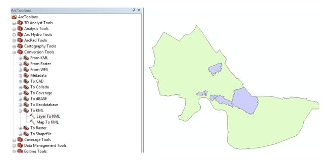
2. Open the ArcToolbox, and navigate to **Conversion Tools.** You'll expand the **To KML** option and select **Layer to KML** to convert your original shapefile into KML format.
