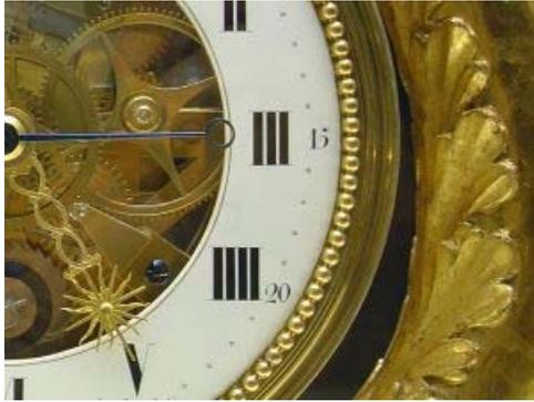
*Clock:* Gears in a clock allow for different hands to turn at different times based on the size of the gears that they are connected to.
