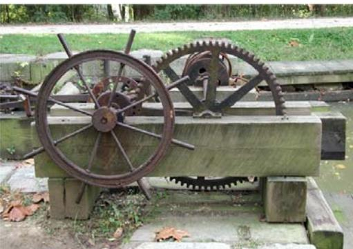
*Drawbridge:* In the olden days, gears were attached to cranks for heavy lifting with high gear ratios, so that with each turn of the wheel, the driven gear only turned a fraction of the way around. This way it was easier to turn the wheel than actually lifting the drawbridge.
