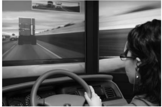
Figure 2. A typical participant conversing on a hands-free cell phone in a three-lane section of the high-flow driving scenario.
