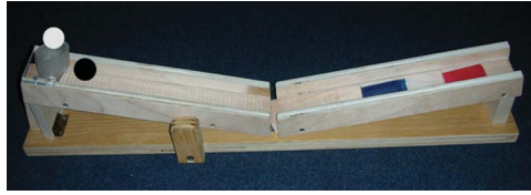
FIGURE 4 Ramp set-up used in Study 2. The height of the downside ramp (left side of Figure) can be raised and lowered. Either a white or black ball can be dropped through the tube to roll down the ramp. The ball can land in either the blue notch or red notch on the upside ramp (right side of figure). (Color figure available online.)
