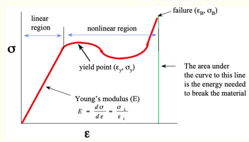
Strain (ε): Amount of deformation of the material in the direction of the force applied. The strain is a dimensionless quantity as it just defines the relative change in shape.
