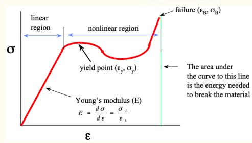
Stress (σ): Force (F) applied per unit area (A). The unit of stress is N/m<sup>2</sup>
