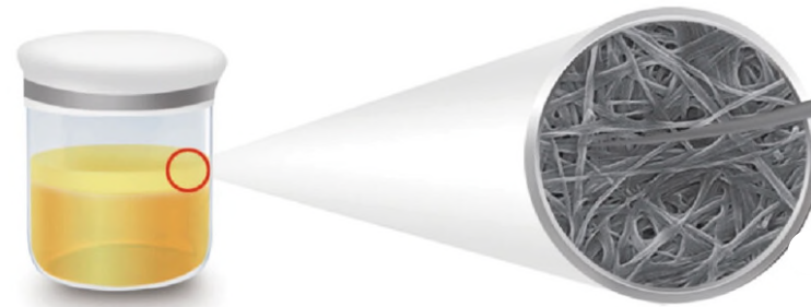
Fiber structural organization in cellulose film
