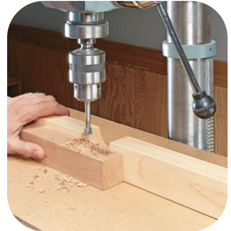
Drill presses can insert holes into pieces
