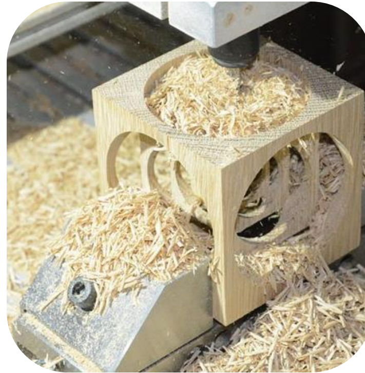
Mills can cut fine, irregular shapes
