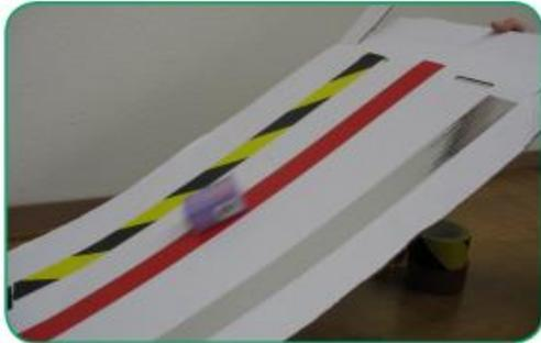
Figure 1. Sample cardboard ramp with different paths made of varying textures to affect friction including: tape, sandpaper, etc.
