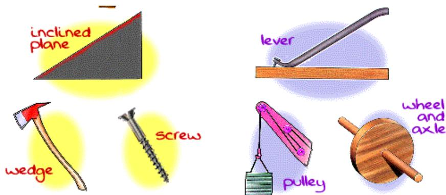
Most of you used **wheels** to help your robotic vehicle move today. The **wheel & axle** is a type of **simple machine**. As you saw with your robotic vehicles, the wheel and axle can move objects across distances.
