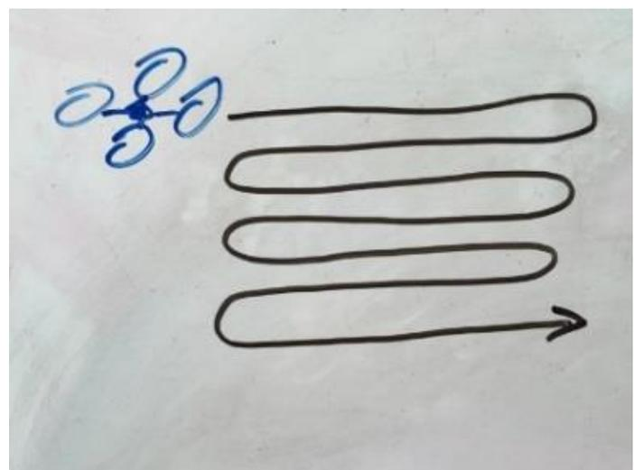
Figure 4. Optimal UAV flight path. This raster pattern allows the UAV to sweep a rectangular aperture.
