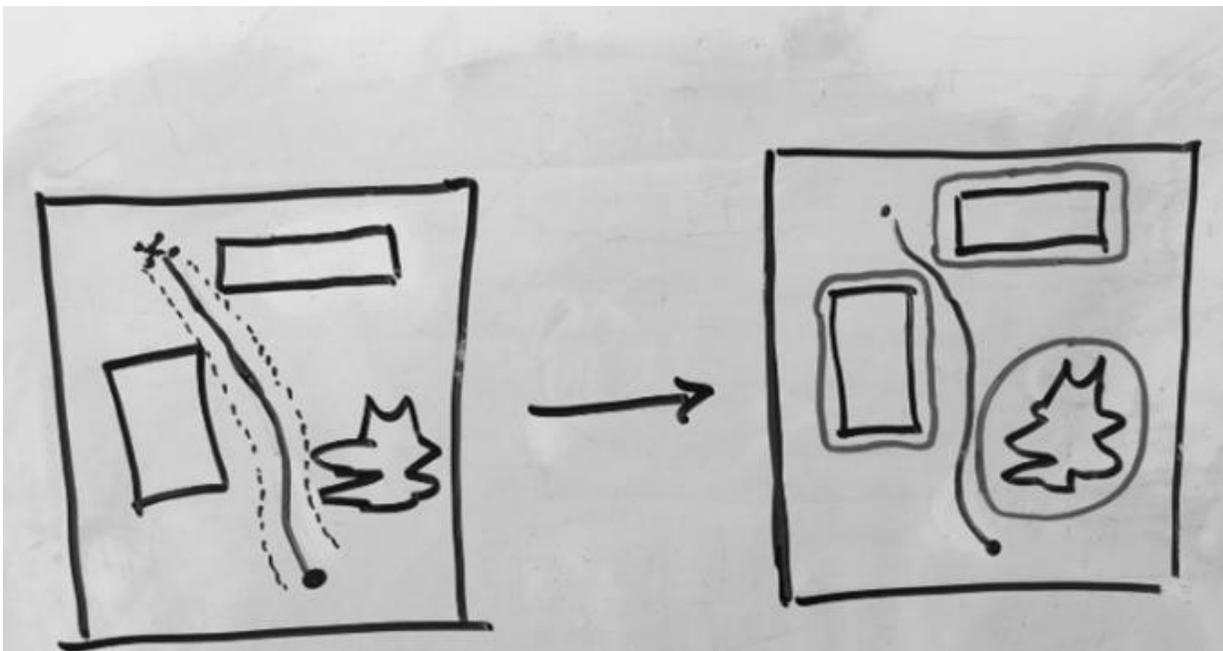
Figure 2: Two path planning sequences. Left: the vehicle is surrounded by a bounding ball. Right: the vehicle is a single point and a buffer radius has been applied to every obstacle.
