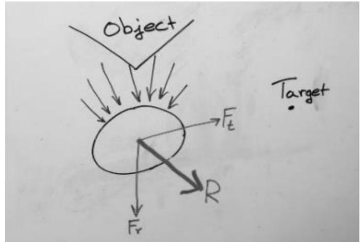
Figure 3. Diagram of the Virtual Force Field algorithm. The object exerts a force on the vehicle, preventing a collision.  $F_r$  represents this repulsive force,  $F_t$  represents the attractive force to the target, and  $R$  is the resultant force.
