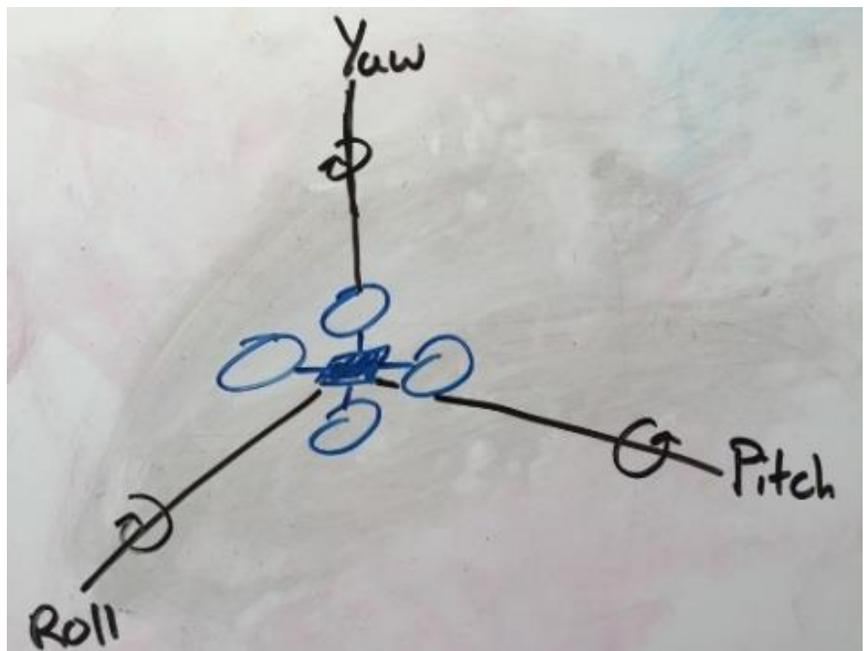
Figure 1: Diagram of Roll / Pitch / Yaw
