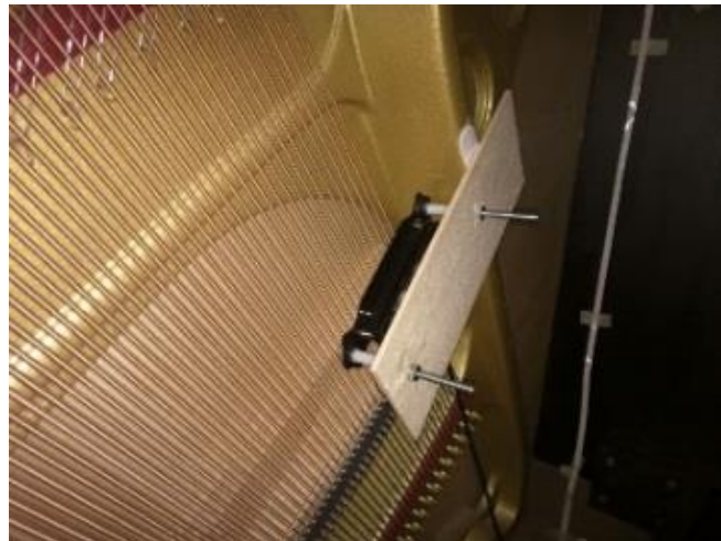
Figure 1: The Rust Team utilized magnetic pickups to convert vibrations of a piano string to an electrical signal. Shown here is a proof of concept version of our device using a guitar pickup to sense a piano note.
