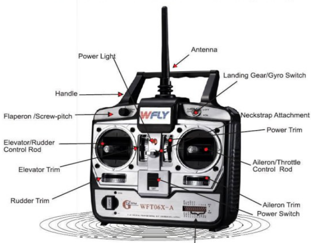
Figure 2. Drone transmitter with universal parts (UAVCoach, n.d.)
