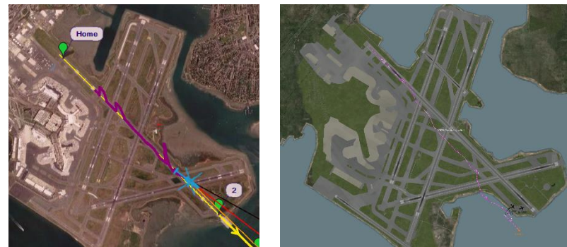
The simulated flight path of a spoofed drone over Boston Logan International Airport. Left: (Purple) Spoofed location experienced by the Drone, (Black) Position Data from Real GPS satellites, (Yellow) Programmed flight path. Right: (Pink) Overlay of actual flight path of the drone.
