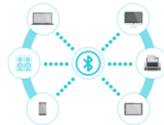
Figure 1: Phones, computers and other devices can be connected through a Bluetooth PAN
