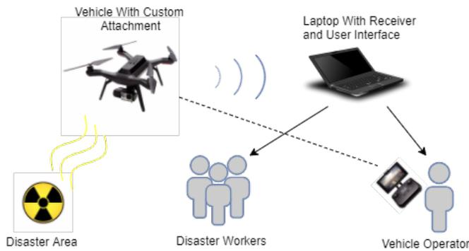
Figure 1: Top-Level System Diagram
