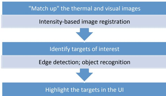
Figure 4: Process Description to Incorporate Thermal Data
