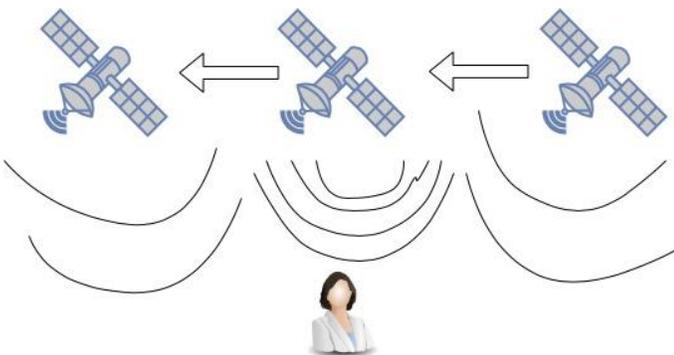
Figure 1: Doppler effect of Sputnik. Frequency of signals increases when the satellite is close to the observer.
