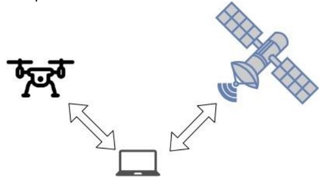
*Figure 2: Direction of communication between satellite, base station (middle), and drone (rover).*
