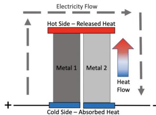
Figure 1. The Basics of Thermoelectrics
