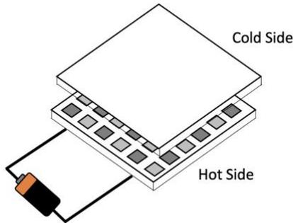
Figure 3: Thermoelectric Module
