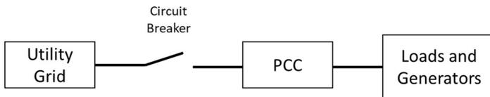
*Figure 2.* The block diagram above represents a microgrid that has been islanded from the utility grid. The circuit breaker has been tripped to disconnect the microgrid from the utilities grid. This disconnection occurs at the point of common coupling (PCC) which is connected to the loads and generators of the microgrid.
