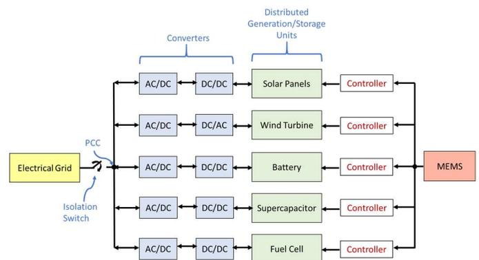
*Figure 1. The block diagram above shows three of the four parts of a microgrid: the distribution network (represented by lines/arrows), the distributed generation units, and the energy storage units. The fourth part, controllable and uncontrollable loads, would be connected somewhere between the PCC (Point of Common Coupling) and the converters.<sup>3</sup>*
