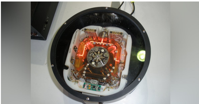
Figure 2. Northrop Grumman Ring Laser Gyro for Submarine Navigation [5]
