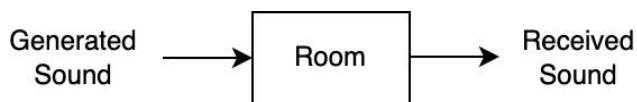
Figure 1. Effect of the room on sound localization represented as a linear system
