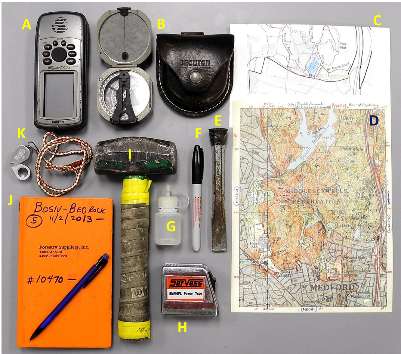
Figure 1.5 – Basic field equipment for geologic mapping: A) GPS device, B) Brunton Compass and case, C) location map for daily mapping agenda, D) map with transparent Mylar sheet glued to it for plotting geologic data locations, E) small chisel, F) permanent marker, G) acid bottle, H) tape measure with metric units, I) rock hammer (small sledgehammer in this case), J) field book and mechanical pencil, and K) hand lens or jeweler’s loupe. Not shown are a camera and clipboard.
