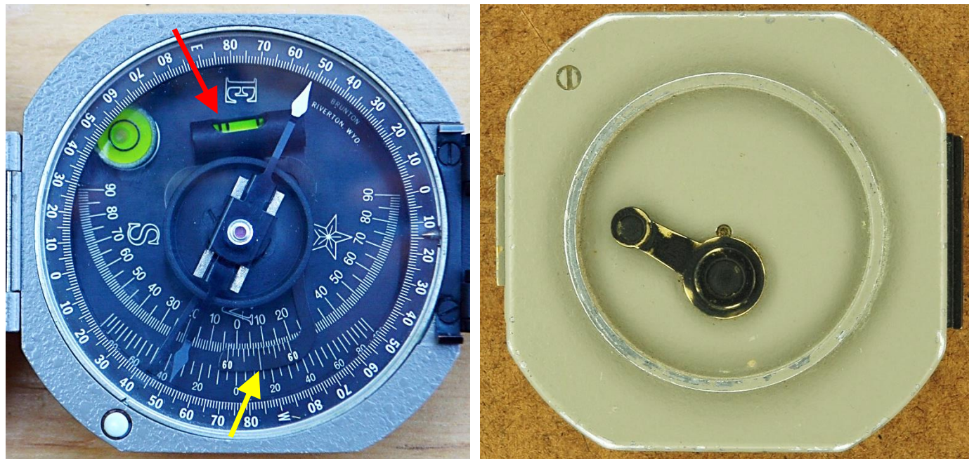
Figure 1.7 – (left) Close up view of Brunton Compass showing inclinometer arm (yellow arrow). Note that the scale on the arm has a center mark (“0” at tip of yellow arrow) that is lined up with 8^\circ on the scale above it indicating the angle (dip) that would be measured when a side of the compass rests on a plane or line dipping at 8^\circ . (right) Back view of Brunton Compass showing lever that is rotated so the inclinometer arm can be leveled (red arrow on front) while one side of the compass housing is resting on a dipping plane.
