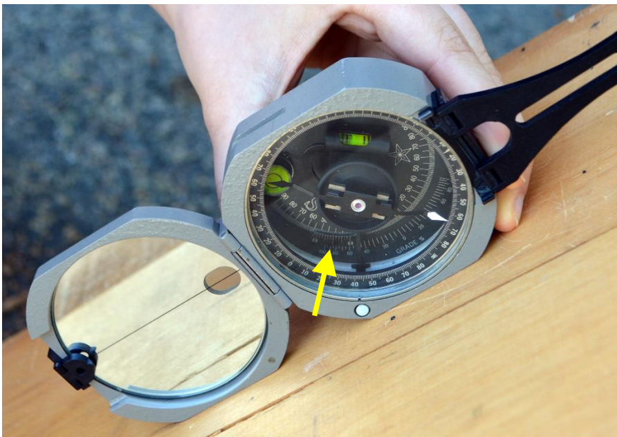
Figure 1.12 – To record the dip of a plane with a Brunton Compass the side of the compass is held against the plane along the trend of the dip, i.e., perpendicular to strike. The inclinometer lever on the back of the compass (Fig. 1.7) is turned until the level on the arm is centered. The scale inside the arm reads the dip in degrees. Here the dip is 41° (arrow). The quadrant of the dip direction should also be recorded as either NE, SE, SW, or NW. The quadrant will be 90° clockwise from the strike direction using the right-hand rule.
