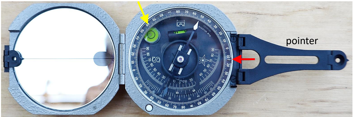
Figure 1.6 – A Brunton Compass which measures compass directions and has an inclinometer for measuring dip angles. The light green circle with a bullseye (yellow arrow) is a spirit level used to horizontally level the compass when measuring directions. The black foldout lever on the right side is the pointer. The scale on the rim of the compass housing is offset by about 14^\circ from the pointer on the compass, i.e., “0” is not aligned with the pointer (red arrow). The scale is turned with a set screw and adjusted for the magnetic declination of the field area. In this case, it is adjusted for a magnetic declination in the Fells of 14.3^\circ\text{W} in 2021. Inside the lid of the compass is a mirror with a view hole (left side) that can be used for sighting on objects.
