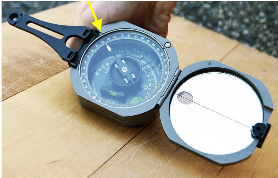
Figure 1.11 – To record the strike of a dipping plane the lower edge of the side of a Brunton Compass is held against the plane (here a tilted wooden box) while the pointer on the compass is pointing in the direction of strike according to the right-hand rule. The view here is looking down on the compass in the downslope direction. When the bullseye level is centered, i.e., the compass is horizontal, the direction of the white end of the compass arrow is recorded. One should be careful in doing this if the rocks you are measuring are magnetic because they can deflect the compass reading. The compass in this image is reading N42°W (arrow).
