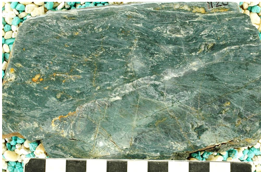
Znmp51: Sheared volcaniclastic rock with domains that were once pebbles. Rock occurs along a fault west of Middle Reservoir in Stoneham (site 11120). Thin section view is in Fig. Znmp50 above.
