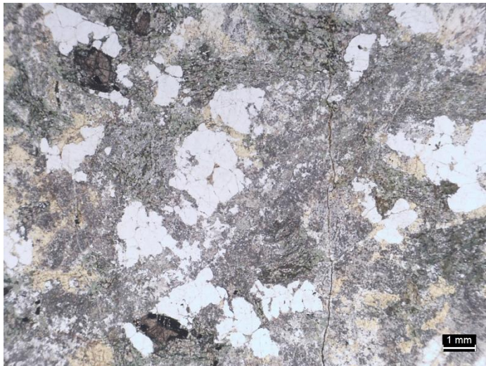
Zwg20: Granodiorite near west end of Hillcrest Parkway (site 11097). Quartz is polycrystalline, alkali feldspar is interstitial, and plagioclase (gray) is heavily altered to sericite. Most mafics are altered to chlorite. Dark high relief mafic grains are sphenes (titanite). (See Fig. Zwg5.)
