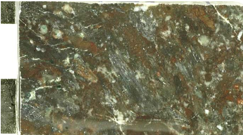
Zlvx13: Dark red to gray, faintly banded crystal tuff at northeast corner of Wrights Pond in Medford (site 10467) with flattened pumice.
