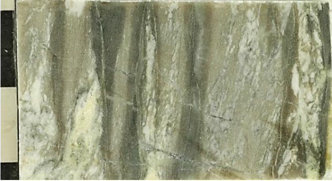
Zvw8: Interlayered, gray fine tremolite-rich quartzite layers with Ca/Mg-silicate zones (white areas with calcite, diopside, and tremolite) that are sheared into small boudins along Pond Street at Spot Pond in Stoneham (site 10316; see Fig. Zvw5 above).
