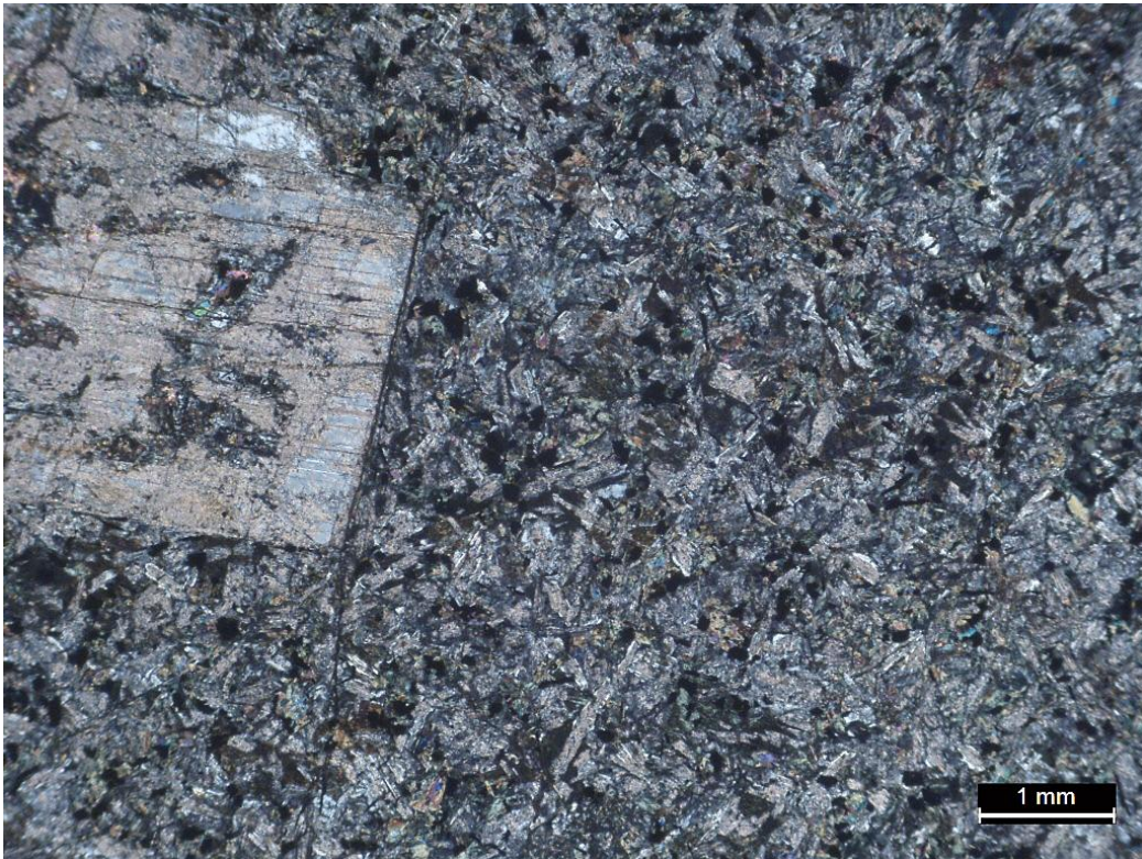
dp17: Porphyritic dolerite dike (dp) cutting through Nanepashemet Formation (Znmp) along west shore of Middle Reservoir in Stoneham (11268). Thin section with crossed polarizers. Fine intergranular texture with a matrix of tabular plagioclase highly altered to sericite and clinopyroxene completely altered to fine chlorite and actinolite. Phenocrysts are very coarse plagioclase heavily altered to sericite and epidote.
