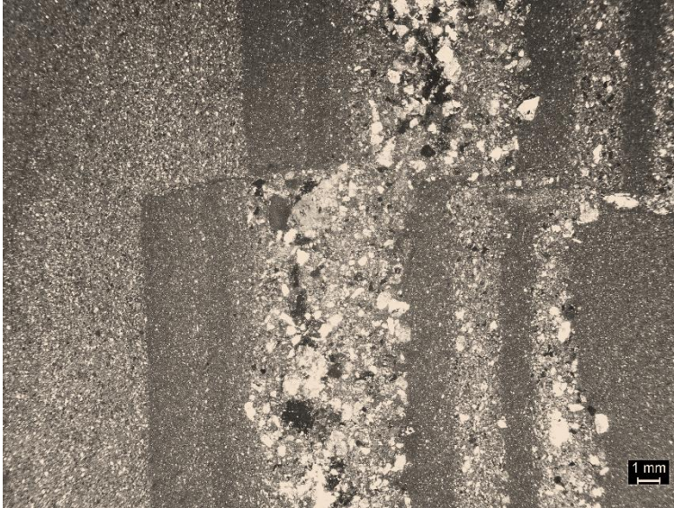
Zvw29: Interlayered argillite and thin sandstone beds with little stretching of original bedding in Pine Banks Park in Melrose (site 11452). Fine-grained matrix material surrounds most larger grains. This site is unusual because it also has many very angular grains. Up is to the left. Silicification at this site is discussed with the Boojum Rock Tuff and unconformity on the Westboro at this site.
