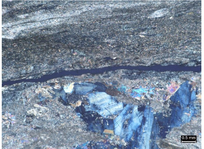
Zvw48 (above): Quartzite and argillite with abundant tremolite, diopside (bright colors in right center) and zoisite (grayish-blue and zoned) on Pond Street in Stoneham (site 11284). See Figs. Zvw11 and 18 for outcrop and cut rock views. Dark line across center of view is an open crack.
