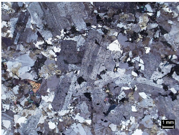
Zlwg26: Patchy equigranular matrix in porphyritic granophyre along Rt. 93 on east side of Pine Hill (site 10981). Note occasional, interstitial granophyric grains. Colorful grains are epidote. Faint tan to yellowish colors are a potassium stain. Thin section with crossed polarizers. See Fig. Zlwg9 for cut rock view.
