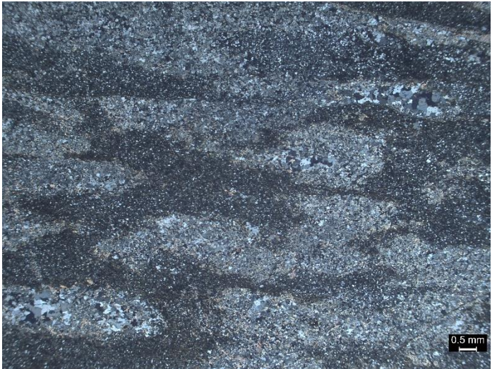
Zvw46 (above): Highly sheared argillite with fine quartzite boudins west of southern South Reservoir in Medford (site 11032). This site sits adjacent to an east-west trending fault that likely contributed to deformation. See Fig. Zvw16 for cut rock view.
