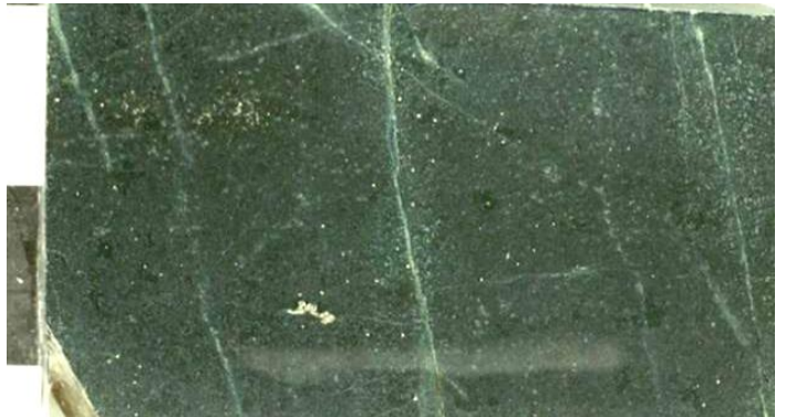
Zlbf3 (left): Cut rock view of relatively coarse porphyritic basalt with oxide veins on Straw Point in Stoneham (site 10603).
