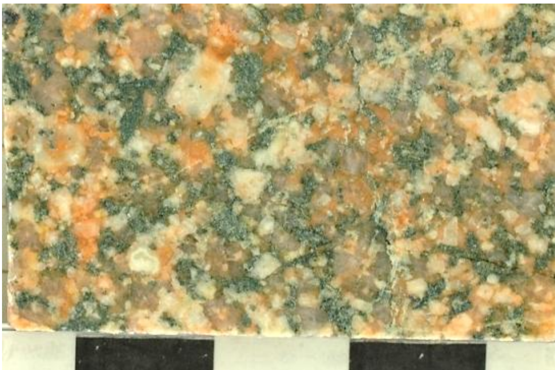
Zwg6: Cut rock slab of granodiorite with orangish-red alkali feldspar at north end of Middle Reservoir near contact with Nanepashemet Formation (Znpm) in Winchester (site 10838).
