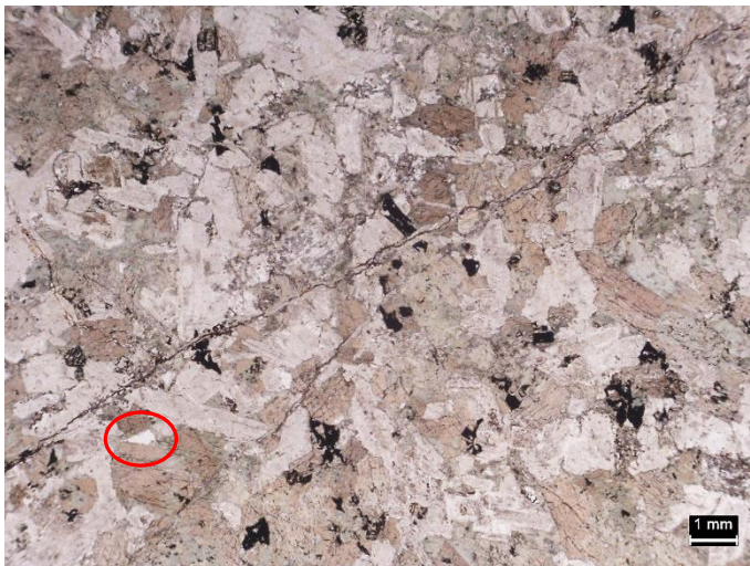
Zdg3: Thin section view in plane polarized light (left) and same image with crossed polarizers (right) of diorite west of South Reservoir in Medford (site 11267). Tan to brown grains are hornblende. In the lower left, the bright grain is rare quartz (circle).
