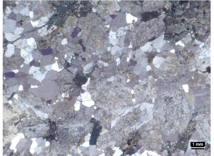
Zwg11: (left in plane polarized light, right with crossed polarizers) Granodiorite north of Long Pond (site 11095). Quartz is polycrystalline, alkali feldspar (stained yellow) is interstitial, and plagioclase is gray due to alteration to sericite and scattered fine epidote. Mafic minerals are hornblende mostly altered to chlorite.
