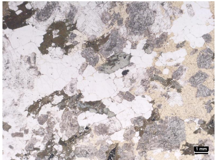
Zwg17: Granodiorite near North Reservoir Dam (site 11230). Quartz is polycrystalline and alkali feldspar (stained yellow) encloses euhedral plagioclase that is gray due to alteration to sericite. Mafic minerals are biotite (dark brown) and hornblende (green) with minor alteration to chlorite.
