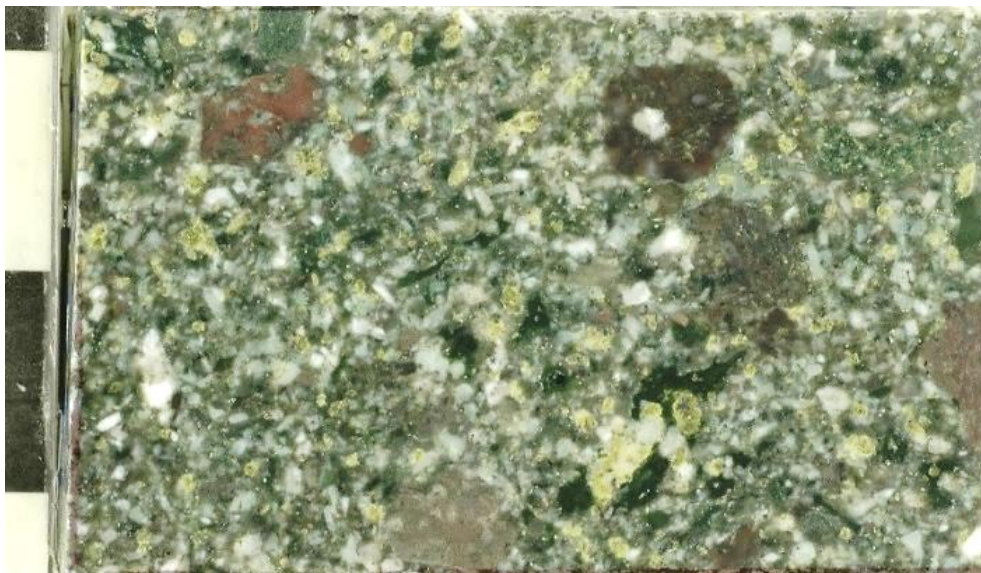
Zbrl4: Lithic crystal tuff west of Black Rock in Melrose (site 10020) with pink and red volcanic lithic fragments and areas of epidote mineralization.
