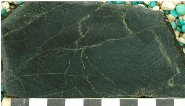
Zlbf2 (right): Cut rock view of altered basalt with quartz and epidote veins at Straw Point in Stoneham (site 10430).
