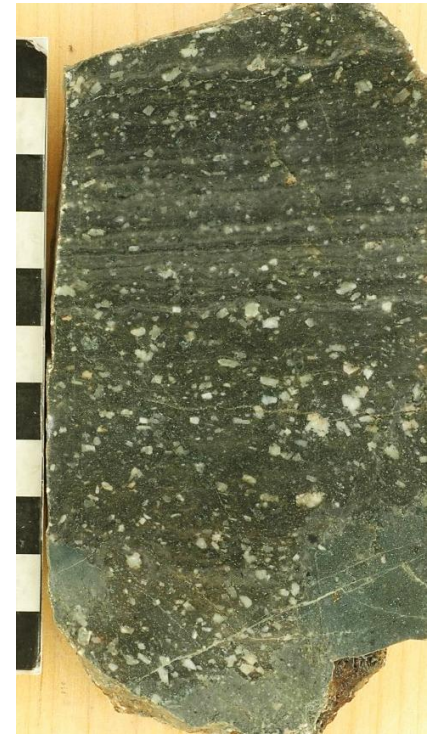
Zlvp3 (right): Well banded rhyolite porphyry near unit's contact (bottom of image) north of Boojum Rock in Stoneham (site 10912). Bands are parallel to contact.
