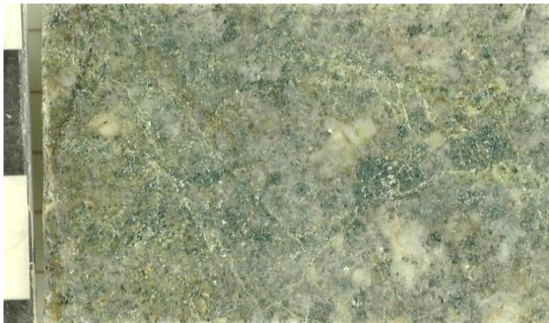
Zst4 (right): Partly assimilated xenolith of the rhyolite flow facies of the Lynn Volcanic Complex (Zlvf) in Stoneham Granodiorite (Zst) chill zone at northwest shore of Spot Pond (site 10422).
