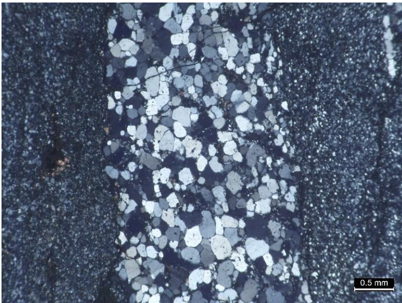
Zwp18: Well sorted and rounded quartz sandstone bed (bedding vertical in image) just above fault contact with the Lynn Volcanic Complex (Zlvx) at the south end of Whip Hill in Stoneham (site 10573). Surrounding the sandstone bed is fine sandstone to siltstone. The quartz grains are rounded and lightly sutured but not polycrystalline. Between the sand grains are silt grains and minor chlorite and sericite.
