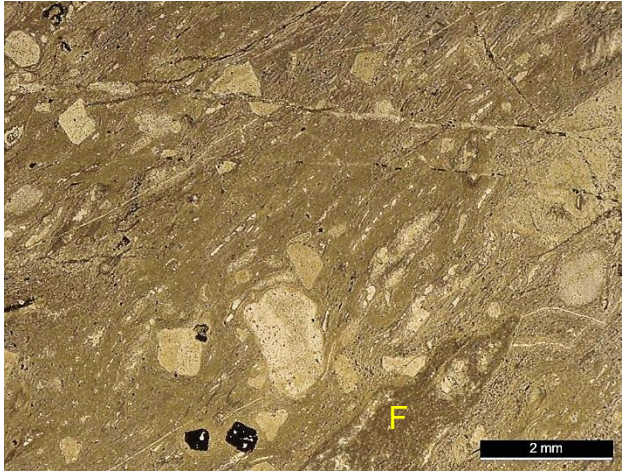
Zlvx16: Banded (lower left to upper right), eutaxitic rhyolitic crystal tuff with broken crystals and flattened glass fragments (light streaks) west of Boojum Rock in Medford (site 10236). Large dark, pinched and flattened fragment near bottom (F) is eutaxitic like the matrix. Thin section in plane polarized light.
