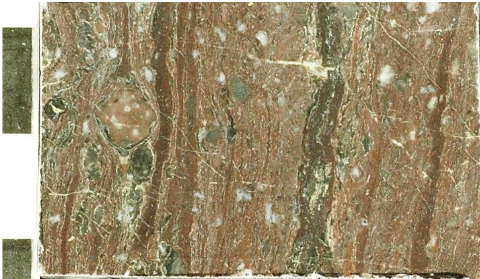
Zlvx5: Rhyolitic welded tuff with pyroclastic banding, crystals, and lithic fragments on western Boojum Rock in Medford (site 10551).
