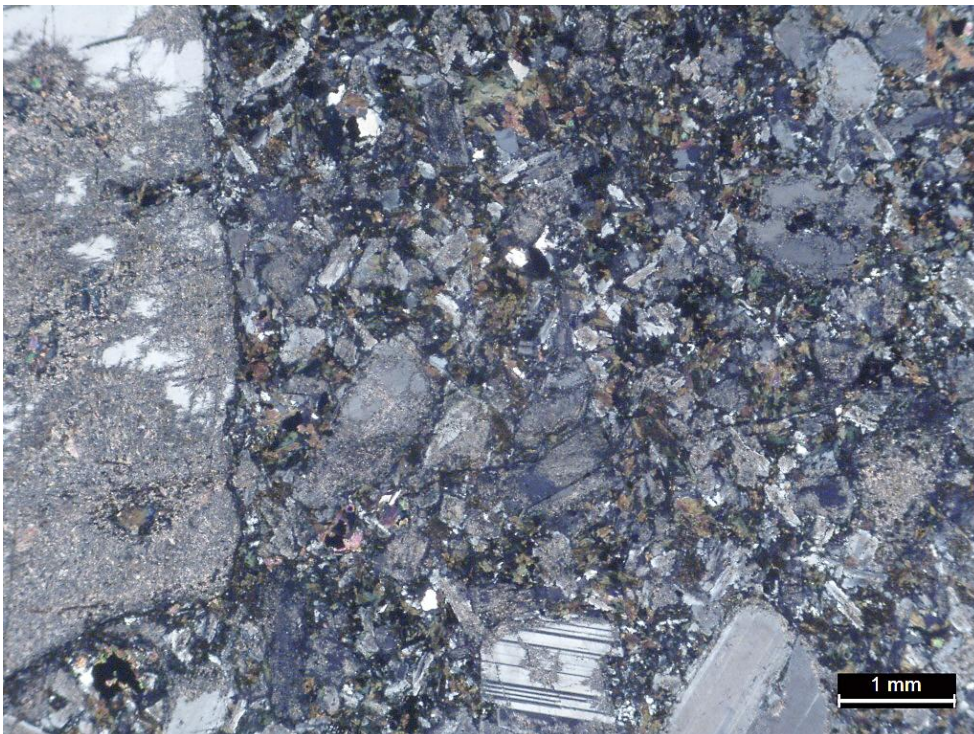
dp20: Porphyritic dolerite dike (dp) in Winchester Granite (Zwg) north of North Reservoir Dam in Winchester (site 11233). Thin section with crossed polarizers. Intergranular texture with tabular plagioclase partly altered to sericite and clinopyroxene altered to chlorite and actinolite. Phenocrysts are plagioclase (left side) irregularly altered to sericite with minor epidote.
