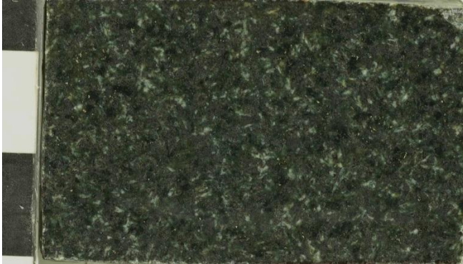
d7: Dolerite dike that is rich in mafic minerals (pyroxene, amphibole, and magnetite) west of Boojum Rock in Malden (site10001).
