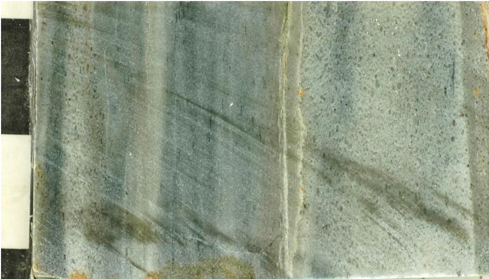
Zvw14: Quartzite layers of varying grain size in Virginia Wood along Spot Pond Brook in Stoneham (site 10297). Quartz grains in the units on the right and far left are flattened and stretched.
