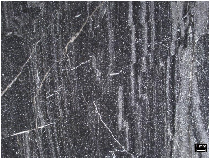
Znpm22: Laminated red sandstone to siltstone in the base of the Nanepashemet Formation along Molly's Spring Road in Medford (site 11068). See Fig. Znpm20 for hand sample view. Thin section in plane polarized light.
