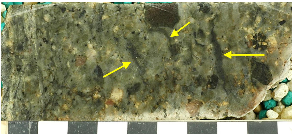
Zlvx70: Light gray weathering crystal tuff with conspicuous volcanic lithic fragments in the conservation land at J.J. Round Park in Wakefield (site 11700). Aligned, flattened glass or pumice fragments (arrows) have a dark color in this rock.
