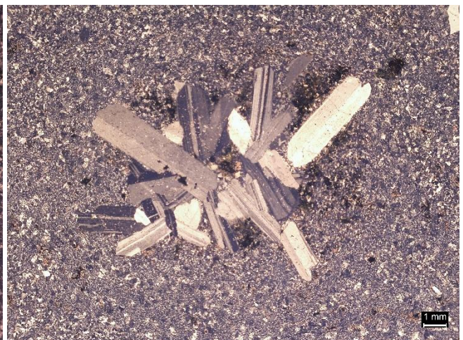
Flow-banded rhyolite on the northwest side of the Fellsway East in Melrose (site 11534). Thin section views with crossed polarizers.
