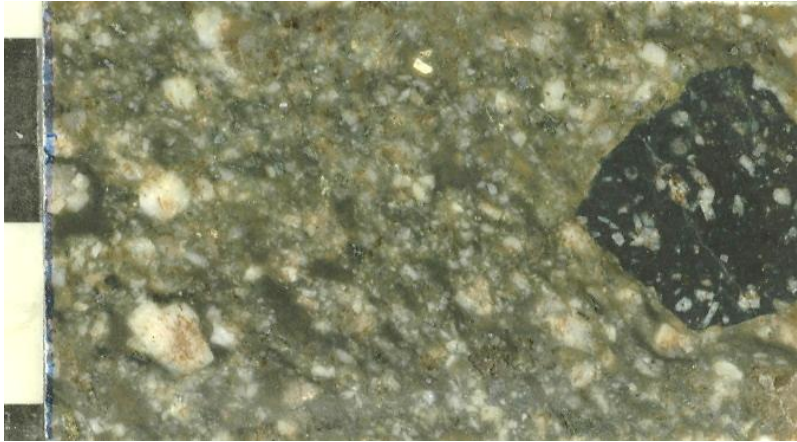
Zlvx35: Welded lithic crystal tuff with fabric (upper left to lower right) formed from dark flattened pumice/glass fragments east of Doleful Pond in Stoneham (site 10407). Note the warping of the dark devitrified glass fragments around the lithic fragment and crystals in the lower right and lower left.
