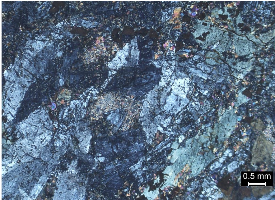
ad9: Dike heavily altered to actinolite and partly recrystallized plagioclase with ilmenite or titanomagnetite altered to the point of slight transparency (dark brown grains near top) on east shore of Middle Reservoir south of Wanapanaquin Hill (site 11155) in Stoneham. View with crossed polarizers.
