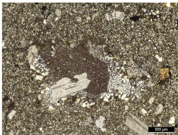
Zlvp8 (above): Granophyric growth on cumuloaphyric plagioclase in rhyolite at south shore of Fells Reservoir in Stoneham (site 10896). Thin section with crossed polarizers. See Fig. Zlvp1 for cut rock view.
