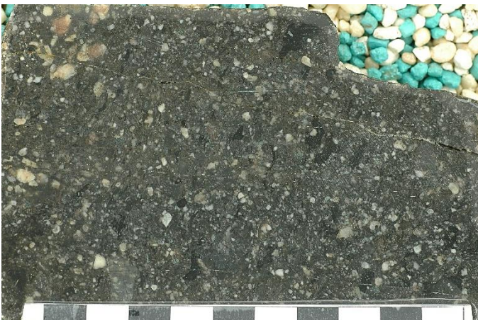
Zlvx37: Welded crystal tuff with embayed quartz xenocrysts and a distinct fabric (upper right to lower left) formed from flattened pumice/glass fragments (black) in Sewall Woods Park in Melrose (site 11537).
