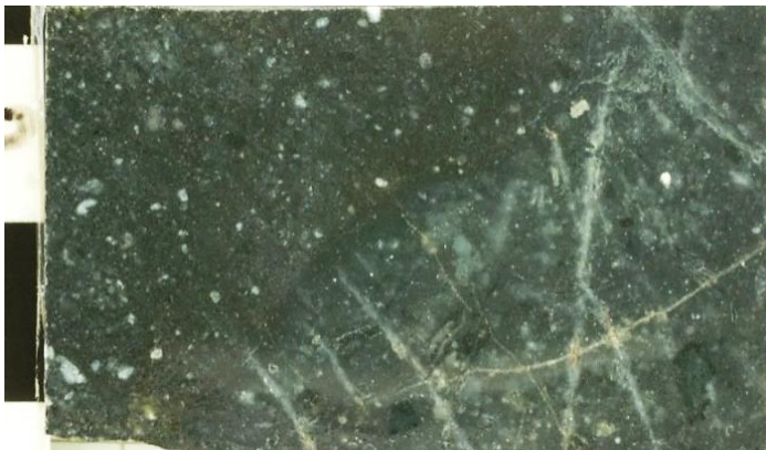
Zlvc1: Volcaniclastic sandy mudstone on northern Pine Hill in Medford (site 10517). This unit shows faint bedding recognized by sand grain abundance and forms the base of the volcaniclastic facies lying on the Spot Pond Granodiorite (Zsg).
