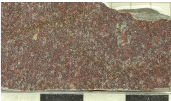
ad5: Cut sample of oxidized dolerite in Fig. ad4.
