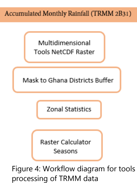
Figure 4: Workflow diagram for tools used in processing of TRMM data
