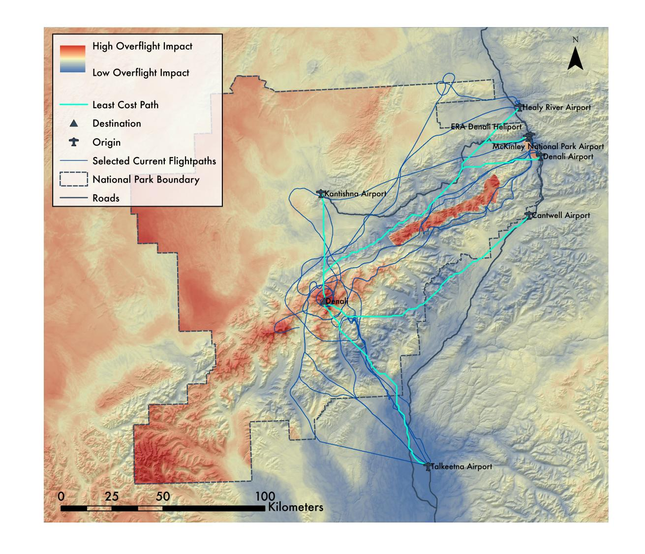
Compared to current routes, optimal flight paths (cyan) avoid areas with greatest noise sensitivity (red), preferring regions with a higher natural ambient noise level (to mask aircraft noise), highest distance from the ground, and least existing opportunities for solitude. This is just one set of paths of the 2,187 possibilities computed by combining the routing factors below in different weighted sums.
