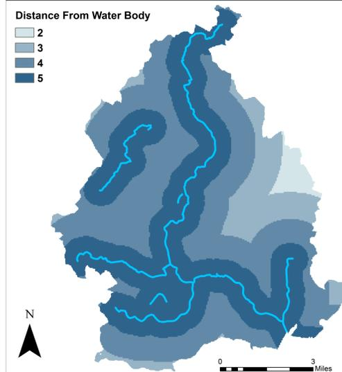
This map considers phosphorus entering the water bodies through stormwater runoff. Stormwater carries high amounts of phosphorus, therefore contributes significantly to phosphorus loading risk. The areas closest to the river load the most phosphorus due to runoff, and are ranked the highest for risk, while the areas furthest from the river are ranked the lowest.
