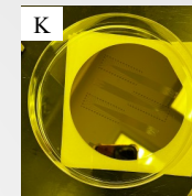
(K) Completed Base Passivation Layer of BioES
