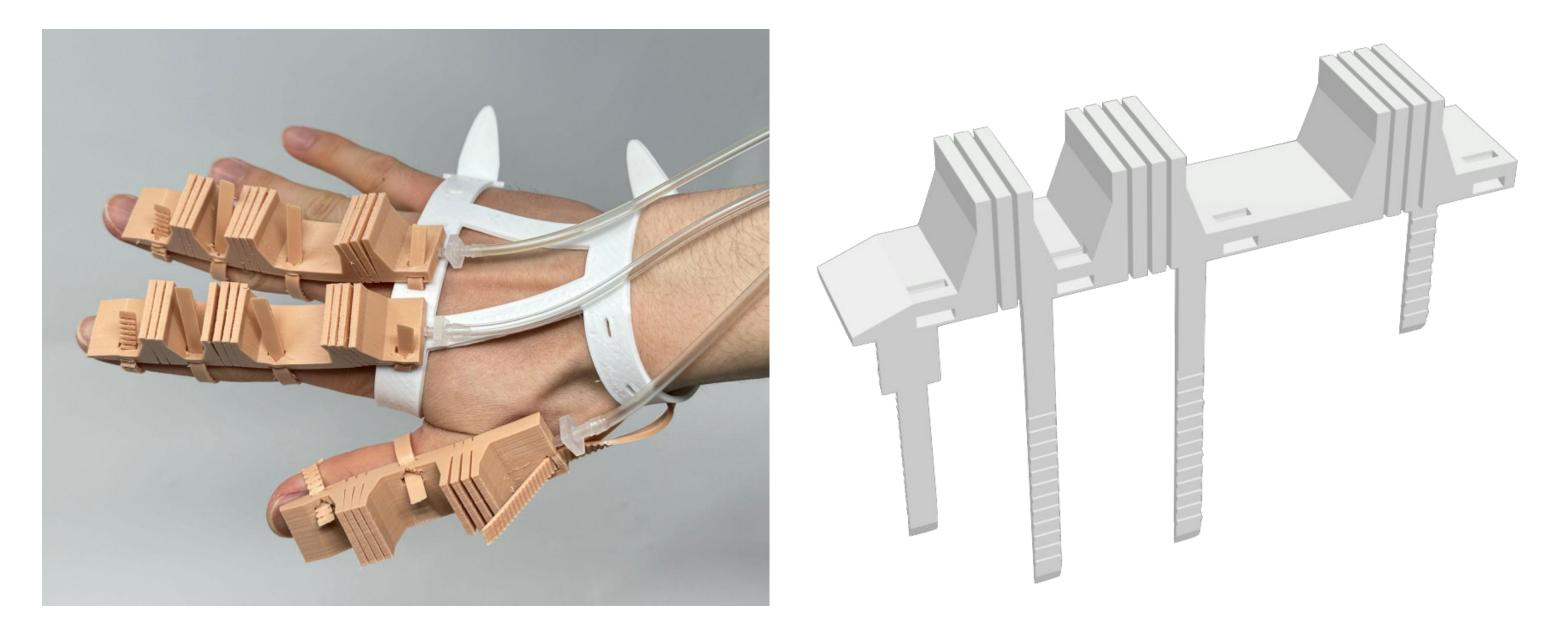
We introduce a design of an exoskeleton that is printable via standard FDM; the design is comprised of pneumatic actuators printed from FilaFlex 60A. It includes printed straps around the palm to connect the exoskeleton to the wrist. Actuators are placed above the MCP, PIP, and DIP to enable flexible extension and bending, while the blocks serve as the skeletal component for
