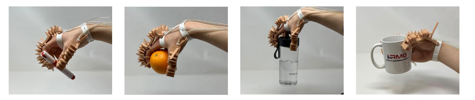
Experiments were conducted with objects requiring different grasp types. The human subject was able to hold objects weighing from approximately 20g to 400g without exerting any voluntary force via finger muscles.
