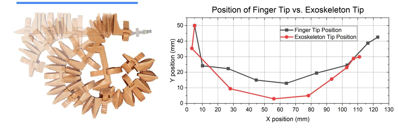
The correspondence between the voluntary movement trajectory of the fingertip and the trajectory of the exoskeleton tip during inflation highlights the alignment with natural human finger movements.
