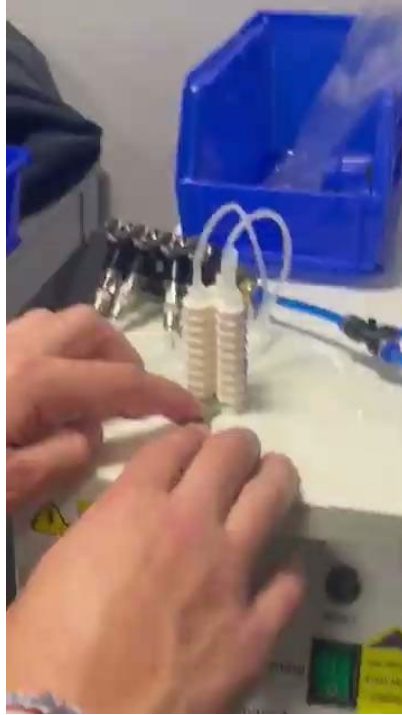
First scaled leg with hexagonal profile: too rigid for 12v pump
