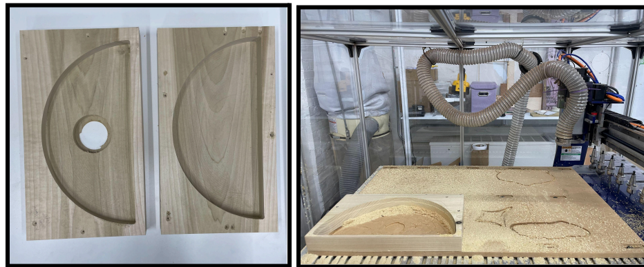
Machine Failure negatives with incorrect cut depth and successful CNC machine bed with negative material
