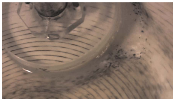
Figure 2. (Color online) A photograph showing the lower half of the wafer and the pepper particle tracers traveling with the slurry flow coming from the bottom right of the image. This image also shows the concentric grooves in the pad becoming clogged with pepper after a long polish.
