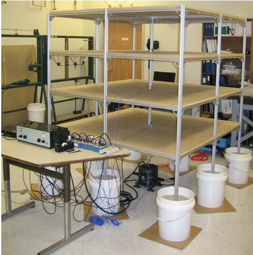
FIGURE 3 THE CONSTRUCTED AND INSTRUMENTED SCALE MODEL BUILDING
