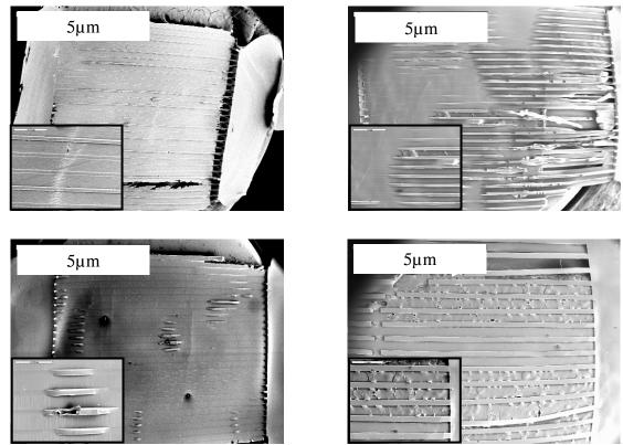
**Figure 3:** Decasted silk films, clockwise from top left, PDMS untreated, PDMS treated for 20 seconds with oxygen plasma, PDMS treated for 20 seconds with oxygen plasma and surface subsequently stripped with a razor blade, and PDMS treated for 20 seconds with oxygen plasma and surface subsequently coated with vacuum grease. Bottom left corner in all images shows a magnified region of a section of the image.
