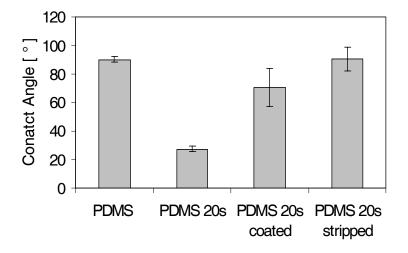
**Figure 2:** The bar graphs indicate contact angle measurements of silk solution droplets on treated and untreated PDMS surfaces (mean value n=3). Black bars indicate standard deviation. *20s* refers to oxygen plasma treatment for duration of 20 seconds. *Coated* refers to a deposited a thin silicone grease film on the surface. *Stripped* refers to removal of the top most layer of PDMS surface with a razor blade.
