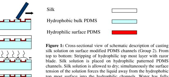
silk solution on surface modified PDMS channels (Group 2). From top to bottom: Stripping of hydrophilic top most layer with razor blade. Silk solution is placed on hydrophilic patterned PDMS channels. Silk solution is allowed to dry; simultaneously the surface tension of the solution forces the liquid away from the hydrophobic top most surface into the hydrophilic channels. Water has fully evaporated and silk fibroin is deposited in the channels.
