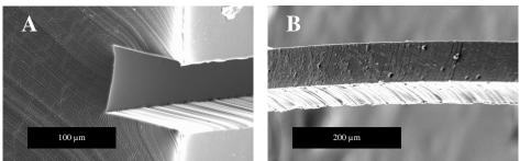
**Figure 4:** SEM image A on the left is showing a PDMS casting channel with width and height dimensions of approximately  $100 \ \mu m \ x \ 100 \ \mu m$ . Image B on the right is showing a single casted silk fiber with the same dimensions.
