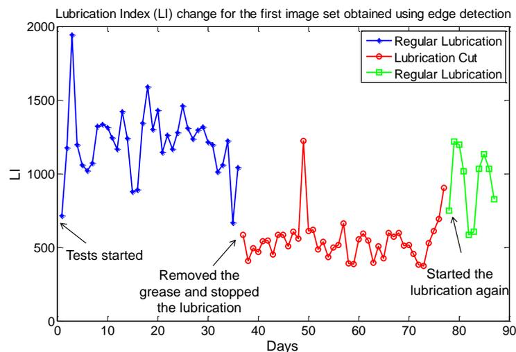
Figure 3. LI for the first image set obtained using edge detection [regular lubrication (baseline), lubrication cut, and regular lubrication (repaired)]
