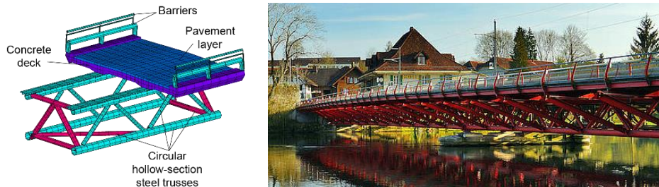
Figure 1: Finite-element model cross-section (left, reprinted with permission from ASCE [3]) and general overview (right) 1 .
