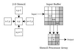
Fig. 10. **Jacobi Stencil** computation performs an average of the cell's Gaussian neighborhood. A single stencil-compute core requires a 3x3 array of elements.  $n^2$  stencil-compute cores require  $(n+2)^2$  elements, i.e. 4 cores requires a 4x4 array of elements, 9 cores a 5x5 array, and so on.
