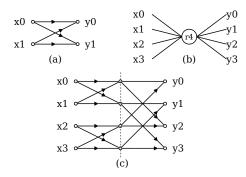
Fig. 6. (a)  $DFT_2$  butterfly operation dataflow. (b)  $DFT_4$  butterfly (c)  $DFT_4$  dataflow composed of two stages of  $DFT_2$  blocks.
