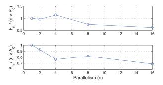
Fig. 4. **DES Parallelism**. Effective power and area cost (y-axis) per core vs. parallelism (x-axis). Naïvely instantiating n cores will cost 1×. Designs with lower cost for high-parallelism are optimal as core-cost is amortized.
