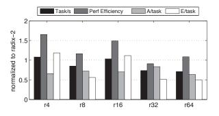
Fig. 7. **DFT**<sub>64</sub> **Core Characteristics.** Performance  $(\frac{task}{s})$ , Performanceefficiency,  $\frac{Area}{Task}$  (area per parallelism in the design), and  $\frac{Energy}{task}$ , varying butterfly-radix from radix-4 to radix-64 normalized to radix-2.
