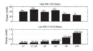
Fig. 5. Use Case: Power for system composed of each design in high-BW and frequency-scaled low-BW use-cases. High BW systems require multiple instances (# shown above each bar). Low BW systems are leakage-dominant with single instance (cycle-time above each bar).
