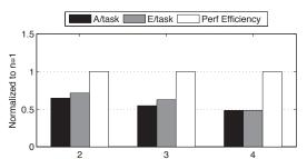
Fig. 11. **Jacobi Core Characteristics.** Area/task, Energy/task and Performance efficiency for n = 2 to n = 4, normalized to baseline n = 1.
