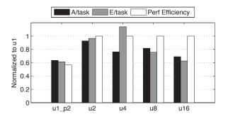
Fig. 3. **DES characteristics.**  $\frac{Area}{Task}$  (Area cost of unrolling, i.e. area per number of logic elements),  $\frac{Energy}{Task}$  (Energy cost of unrolling), and Performance-efficiency normalized to the baseline iterative *u1* DES core.
