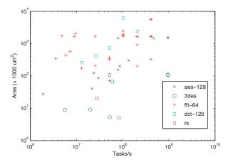
Fig. 1. Area vs. Performance (tasks/s) for fixed-function accelerator cores synthesized from OpenCores[8] and Spiral DSP Framework [9]. Optimal designs are low area (y-axis) and high throughput (x-axis).
