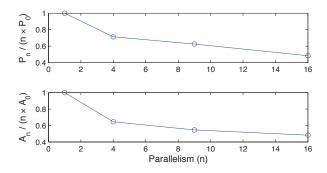
Fig. 12. **Jacobi Parallelism**. Power and Area vs. parallelism, varying the number of stencil cores compared to baseline single-stencil design. Na: ively instantiating n cores will cost 1×. Designs with lower cost are optimal.
