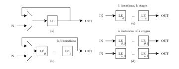
Fig. 2. Dataflow Types: (a) iterative (b) partially unrolled (c) fully unrolled (d) replicated for  $n \times$  streaming throughput
