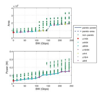
Fig. 9. **FFT-DES Design Space**: Area(top) and Power (bottom) of combined DES-FFT core while sweeping BW constraints. When necessary, each design is frequency-scaled and instantiated multiple times to meet, but not exceed the constraints.
