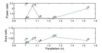
Fig. 8. **DFT Parallelism**. Power and Area cost vs. parallelism (pipeline-depth) for each DFT core, normalized to R64 which has the shallowest pipeline and lowest number of tasks in flight per-cycle.
