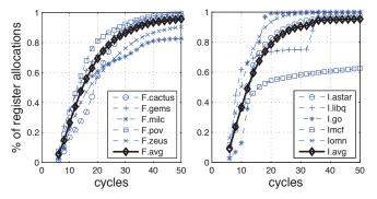
Fig. 2. **"Allocate-write distance"** CDF showing distance between register allocation at rename (cycle 0) and register use at writeback.
