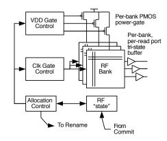
Fig. 4. **Banked Register File**: A partitioned RF allows for modular control of allocation, clock-gating, and VDD-gating when RF state is kept on a per-bank basis. Register reference counts monitor the RF and allow us to implement various allocation algorithms.
