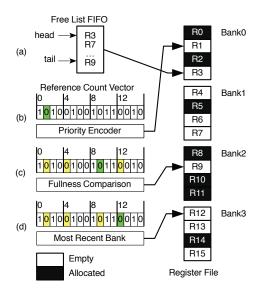
Fig. 3. Allocation algorithms. Each algorithm examines the set of available registers to select the next register for allocation. (a) Free-list: selects the reg at the head of the FIFO queue. (b) Prio: select first free reg from a bitvector representation of the RF ('0'=free, '1'=allocated). (c) Full: select first free reg from fullest RF bank. (d) MRA: select first free reg from most-recently-selected bank
