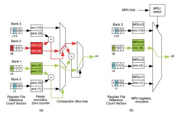
Fig. 7. (a) Fullness Allocation: Zero-counter blocks drive a comparatormux tree propagating the lowest nonzero count and the corresponding register signifier. Bank1 is the fullest bank with only 1 free register, R4 is propagated as the next allocation. (b) MRU Allocation: MRU registers keep track of position in MRU stack. The MRU RF bank with an available slot is selected.
