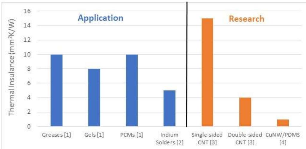
Figure 1 Thermal Resistance of Thermal Interface Materials
