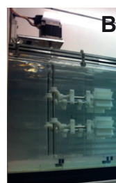
Fig. 1. Experimental setup for respirometry and kinematics experiments. (A) Schematic representation of the experimental design. Turbines are shown in gray with green arrows to indicate rotation. Streamwise vortices and mean flow are shown with blue arrows. (B) Detail of the turbine array.
